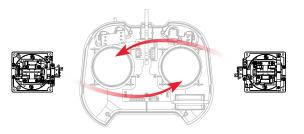
5. Reattach the front cover and back cover, and tighten the screws.
