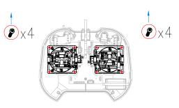
4. Switch the gimbals to the oppsite side and make sure the gimbals have been rotated 180 degrees, then tighten the srcews removed before.
