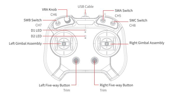
Note: The SWB and SWC switches are for the simulator which includes 8-channel.
