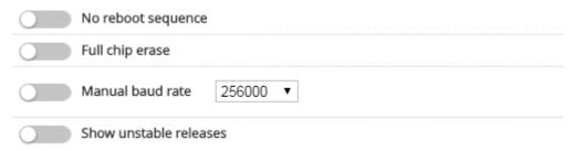
$8. click "Load Firmware [Local]" Select the firmware "betaflight\_3.1.*-3.2-*\_OMNIBUSF4.hex" \ (The firmware version according to the actual situation)$
