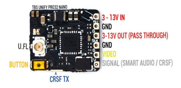
The UNIFY PRO32 5G8 Nano comes with pre installed silicon wires for easy installation in your build. There is a filtered 3-13V input with a pass through output for your camera or other devices.
