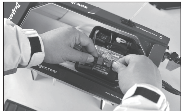
5. Connect the charged Li-po battery to the ESC. The special tone “1 2 3”, 3 short beep then a long “beep” tone are emitted.
